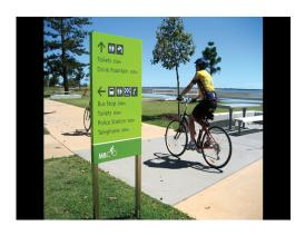
**Turn Signs** indicate where a bikeway turns from one street onto another street. Can be used with pavement markings. Typically placed near-side of intersections and where bike routes turn. Pavement markings can also indicate the need to turn to the bicyclist.
